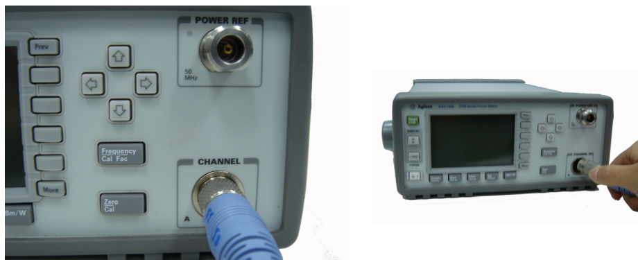
Figure 1-2 Connecting a sensor cable to power meter
